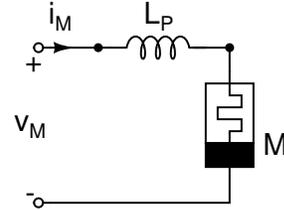
Fig. 3.  $L_P$  is parasitic inductor that is in series with the memristor M.
