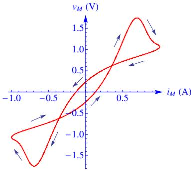
Fig. 7. Mathematica  $v_M - i_M$  for capacitor in parallel with memristor (discharge tube). A parasitic capacitance of 1 F was used, memristor parameters are the same as in Fig. 5.
