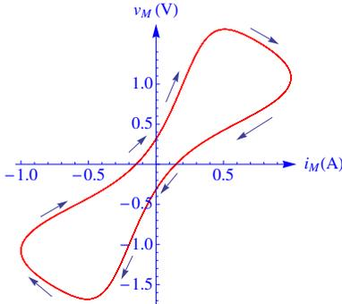
Fig. 6. Mathematica  $v_M - i_M$  for inductor in series with memristor (discharge tube). A parasitic inductance of 5 H was used, memristor parameters are the same as in Fig. 5.
