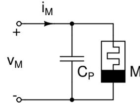
Fig. 4.  $C_P$  is parasitic capacitor that is in parallel with the memristor M.
