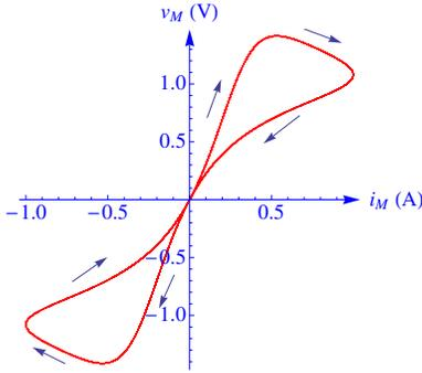
Fig. 5. Theoretical  $v_M - i_M$  memristor (discharge tube) Lissajous figure from Mathematica. Parameters used for simulation were  $\beta = 0.1$ ,  $\alpha = 0.1$ ,  $F = 1$ ,  $\omega = 0.063$ .
