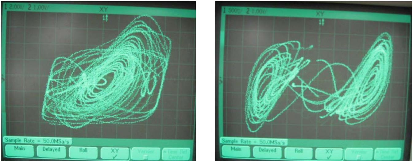
Fig. 8. Two attractors from the physical circuit. The plot on the left is  $v_2(t)$  versus  $v_1(t)$  and the plot on the right is  $v_2(t)$  versus  $\phi(t)$ . The scales for the left plot are 2.00 V/div for  $X$  and 1.00 V/div for  $Y$ . The scales for the plot on the right are 0.5 V/div for  $X$  and 1.00 V/div for  $Y$ . Notice that the plot on the right is in excellent visual agreement with corresponding plot in the simulation (Fig. 4). The plot on the left has some distortion.
