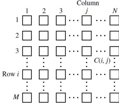
Fig. 1.  $M \times N$  CNN architecture.
