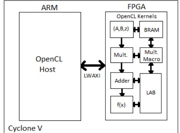
Fig. 3. A high level block diagram of our DTCNN implementation on the Cyclone V. The OpenCL kernels on the FPGA are executed in parallel over an  $r$  neighbourhood. The host process on the ARM core(s) coordinates kernel execution on the FPGA via the LWAXI (LightWeight Advanced eXtensible Interface). Not shown in the block diagram are external peripheral interfaces (such as VGA, for visualizing spiral wave dynamics in Fig. 4).
