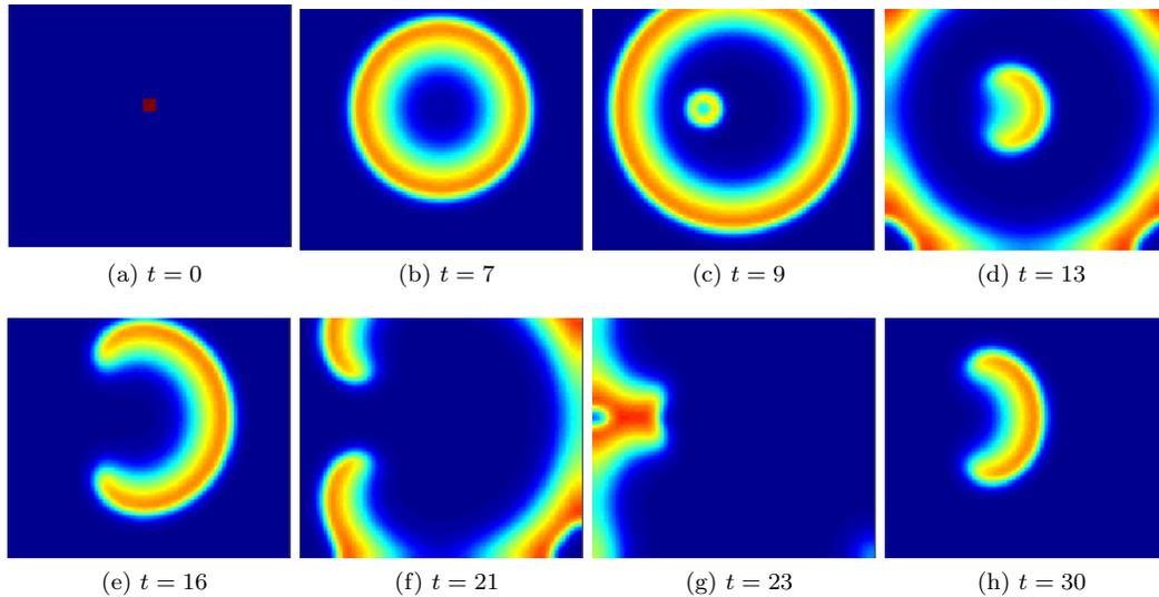
Fig. 4. Spiral wave results from DTCNN specification of FN model. We have used a  $256 \times 256$  CNN and the VGA output is appropriately scaled. One can infer the onset of spiral wave activity at  $t = 13$ . In the given window, the two foci of the spiral wave collide and the pattern from  $t = 13$  repeats at  $t \approx 30$ .
