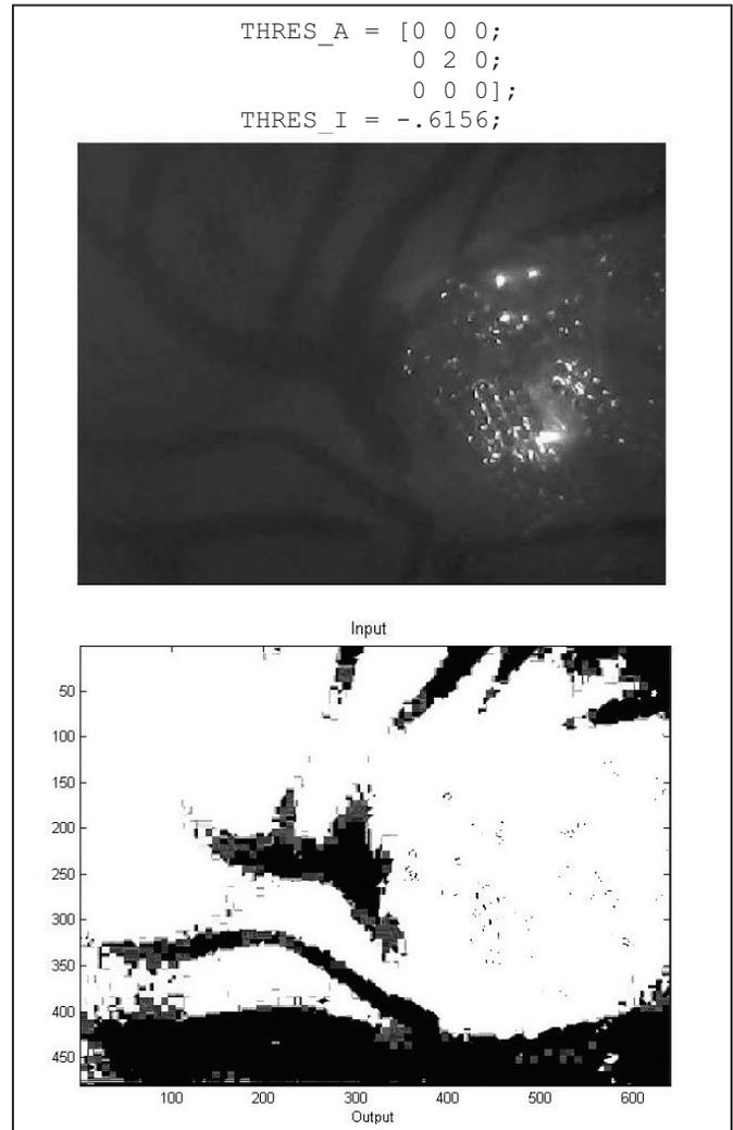
Fig. 1 Threshold CNN template used by *MatCNN*. *THRES\_A* defines the neighborhood feedback, and *THRES\_I* defines the threshold value. The top image is a grayscale photo of a model retina that displays signs of ROP. The bottom image is the output from the *MatCNN* simulation using the threshold template. As shown, the blood vessels were successfully differentiated from their surroundings.
