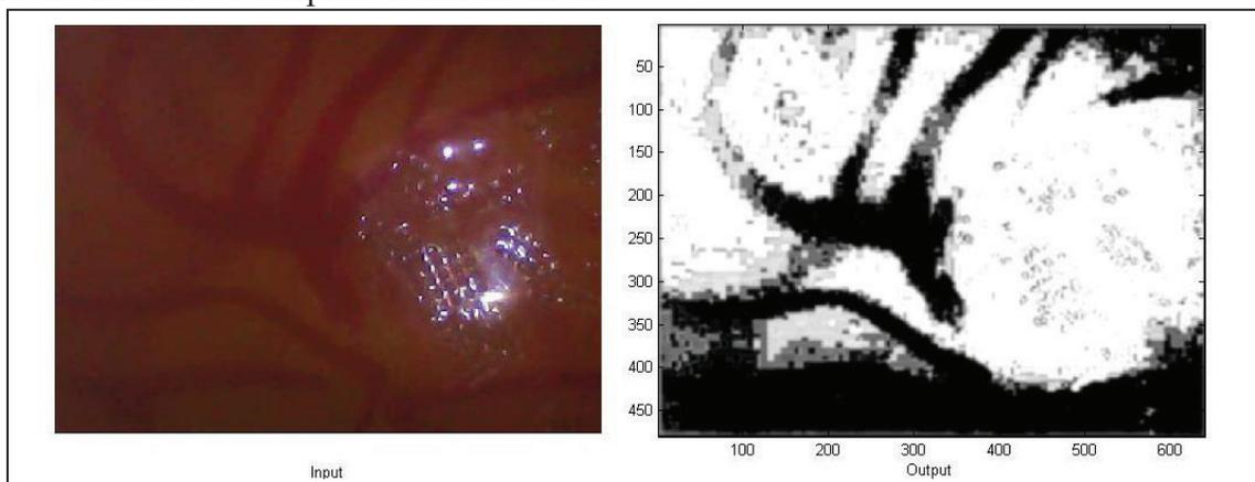
Fig. 2 Final results from the MatCNN simulation. The simulation processed the JPEG image of a model retina (left) through the series of templates described in Section III Subsection B and resulted in the image on the right.
