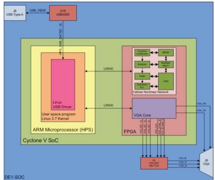
Fig. 3 The block diagram for realizing an FPGA-SoC based CNN image processor to be used for the diagnosis of ROP.
